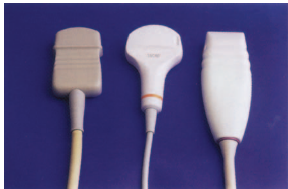
Figure 1.11 Curved arrays (left and centre) suitable for abdominal scanning. A 5 MHz linear array (right) is useful for superficial structures, e.g. gallbladder and anterior abdominal wall.
